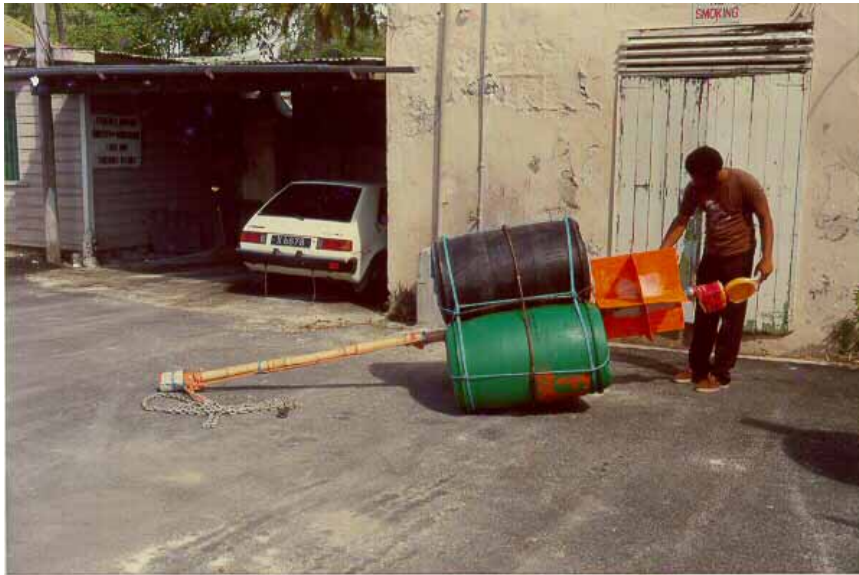
Figure 2: Surface portion of experimental FAD showing arrangement of drums for floatation, radar reflector and light beacon.
